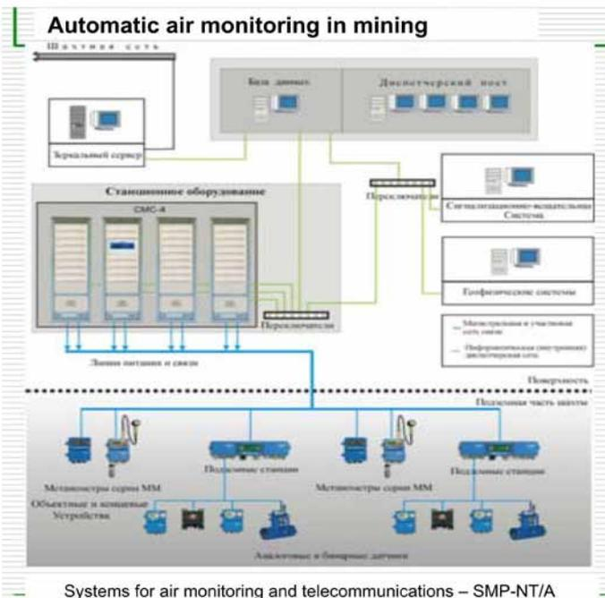
Picture 10. Example of systems of automatic monitoring of geospherical threats.
